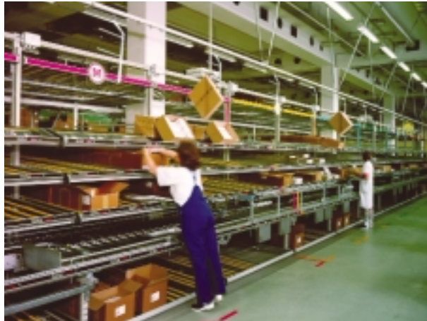
Photo K.9.3. Using "ant": paperless order- picking via Pick by Light
