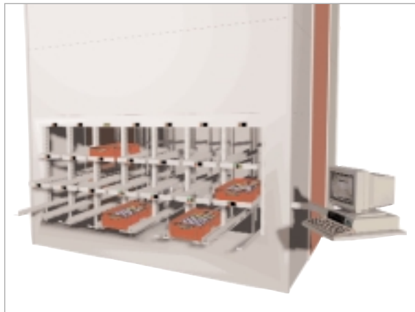
Photo K.9.4. Use in the fully automated high- bay warehouse and in the auto- matic small parts storage system, minilo- ad,
